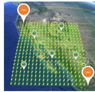
Figure 1: This 8-connected graph was used as the underlying graph for all experiments. The weather locations are marked with green markers and start and goal locations are marked with orange markers.
