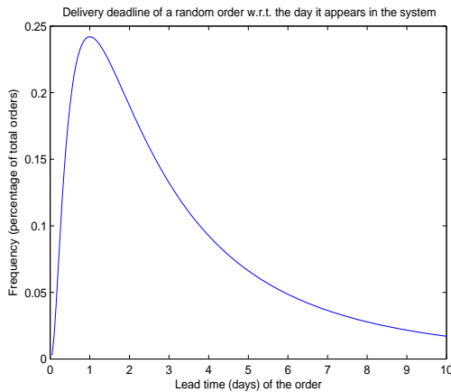
Figure 1: Example distribution of delivery deadlines for orders, in number of days from the present time, for a load with minimum lead time of 1. The date when an order appears in the system corresponds to the origin.
