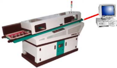
Figure 1. Old machine design: The processing units (modules) are contained within one static monolithic block and centrally controlled.
