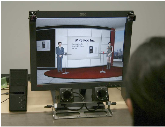
Figure 4: System setup with stereo cameras of the eye tracker in the front, and two infrared pods attached at top of the screen.
