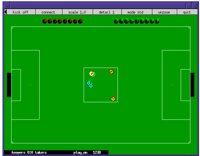
Figure 2: This figure shows a screenshot of the visualizer used for the human to demonstrate a policy in 3 vs. 2 Keepaway. The human controls the keeper with the ball (shown as a hollow white circle) by telling the agent when, and to whom, to pass. When no input is received, the keeper with the ball executes the Hold action, attempting to maintain possession of the ball.
