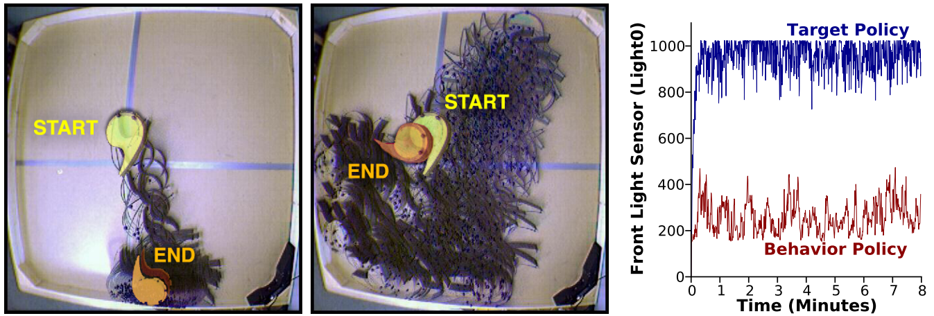
Figure 6. Learning light-seeking behavior from random behavior. Shown are superimposed images of robot positions: Left) In testing, the robot under control of the demon policy turns and drives straight to the light source at the bottom of the image; Middle) Under control of the random behavior policy for the same amount of time, the robot instead wanders all over the pen; Right) Light sensor readings averaged over seven such pairs of runs, showing much higher values for the learned target policy.
