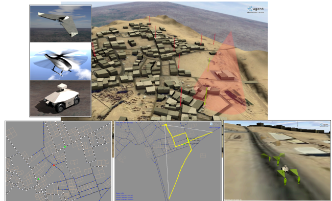
Figure 1: Tactical AgentScout simulator facilitates rich models of physical reality and supports physical mobility dynamics of robots, such as ground and aerial vehicles, be it fixed-wing aircraft, helicopters or various rotorcraft.
