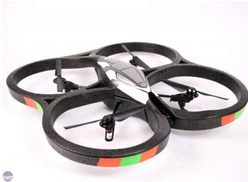
Figure 1 Parrot AR Drone v1.0 with Orange Tags
