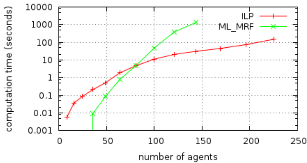
Figure 2: Computation average times for the PNE problem in square grids made of 2 actions agents.
