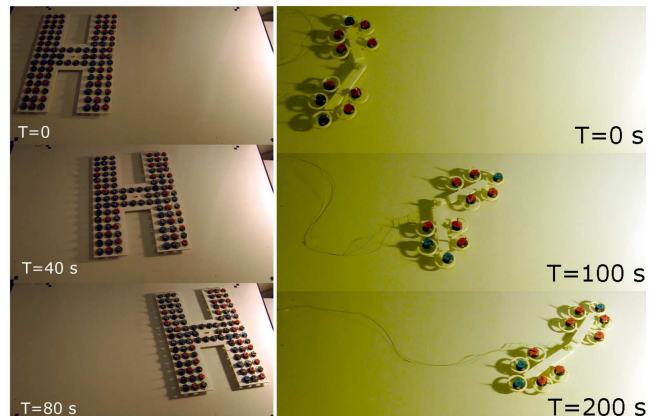
Figure 1: (Left) 100 robots transporting an “H” object. (Right) Kilobots transporting an actively moving object.
