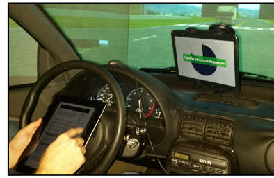
Figure 1: Semi-autonomous vehicle simulator: System requests to transfer control to a busy driver.
