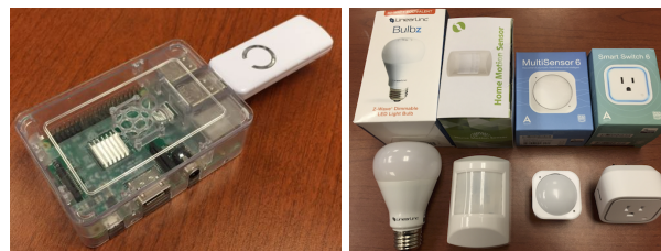
Figure 3: A Raspberry Pi with Z-Wave Dongle (left); Example of Z-wave Compatible Smart Devices (right)
