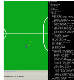
Figure 2: The SRTR tool. Main panel visualizes world state, right panel is a log of internal state, and bottom drop down box selection of desired transition.
