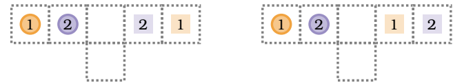
Figure 1: Example where task assignment and path planning cannot be decoupled for the optimal solution. Start positions are circles and goals are squares. Left: Robot 2 must move into the alley temporarily, resulting in a total cost of 8. Right: Both robots can move along their direct path without collision, resulting in a total cost of 6.
