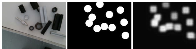
Figure 9: Left: An example haystack image from the evaluation set. Center: The ground truth, approximated segmentation for learning Task 2, i.e., all filters are active. Right: The segmentation output of the network.
