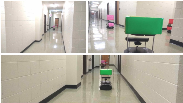
Figure 5: In counterclockwise direction: patrollers (in pink and red) in the longer hallway. Learner (green) observing them from its vantage point in the smaller hallway, and learner breaching patrol to reach the goal (first door to its right).
