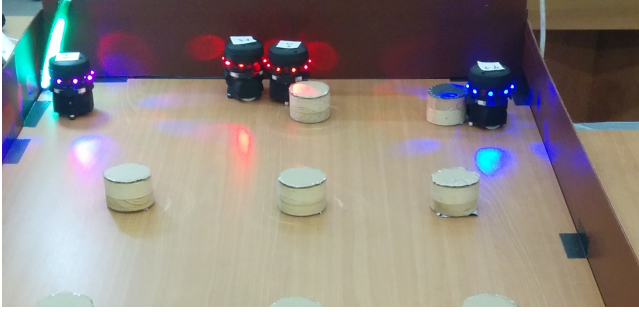
Figure 2: Krembot swarm robots.
