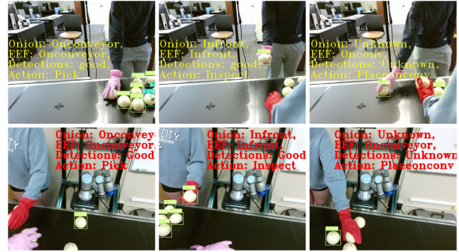
Figure 5: Some of the image frames that compose the joint state-action trajectories \mathcal{X}^E via SA-Net [31]. The annotations on the images are the state-action predictions and the bounding boxes are generated by YOLOv5. The first frame captures when the onion is on the conveyor and the human expert is about to pick. The second captures the human inspecting and finding a good onion. The third is when the human is placing the onion back on the conveyor.
