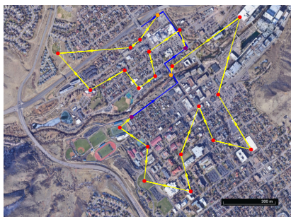
Figure 5: UAV path generated using MINLP approach for a case study in an urban environment.
