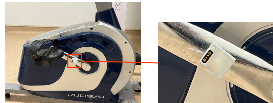
Figure 2: A custom-made speed-sensing unit mounted on a stationary bike.
