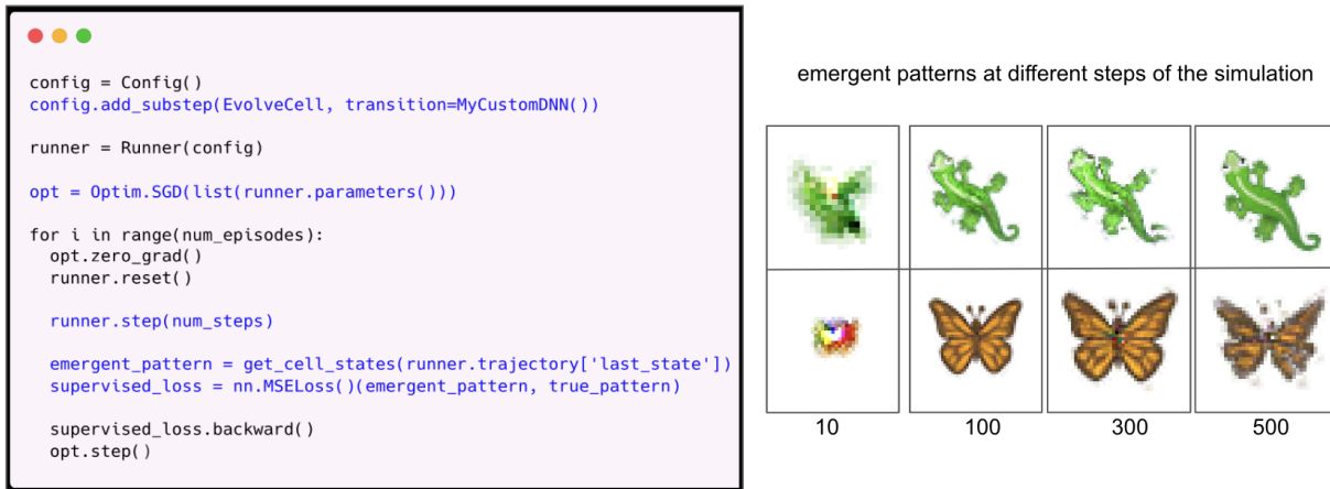
Figure 3: C1: Embed DNN inside ABM with flame. [32] uses cellular automata to simulate morphogenesis and parameterizes the update rules with a CNN. flame is used to learn these rules by representing the substep transition function with a DNN (MyCustomDNN()) and optimizing with an MSE loss (supervised_loss). Enabling this requires only a few additional lines, as shown in the pseudocode on the left, and is an instance of Mode 2 in sec 3.6. Result, on the right, shows the emergent pattern for two shapes (lizard and butterfly) at different steps along the simulation.
